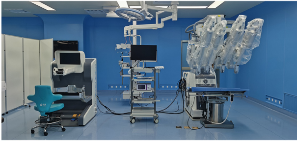
Figure 1 Components of the SHURUI system (Beijing Surgeri Technology Co., Ltd., Beijing, China). The SHURUI system comprises a surgeon console, a vision cart, and a patient-side cart (from left to right).
