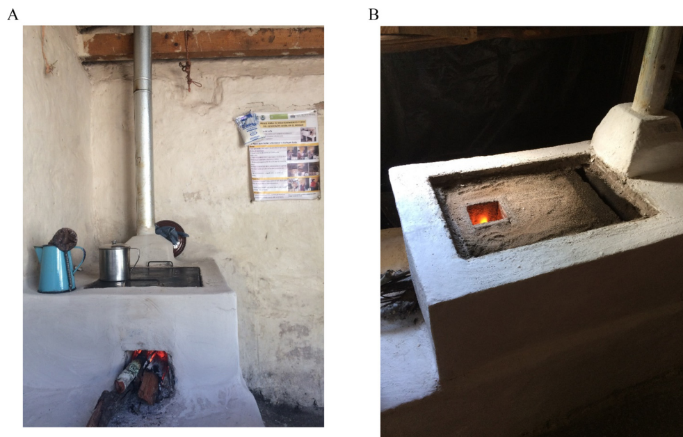
Figure 2. Examples of Justa cookstoves showing an external view preparing coffee (A) and an internal view with the griddle removed (B). Photo credits: Bonnie Young.
