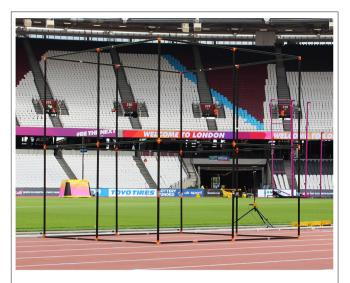
**FIGURE 1** | Calibration frame used in the current study (3.044 m³). The calibration frame pictured was placed at various locations across and along the running track, ensuring the full hurdle clearance was calibrated for each athlete.
