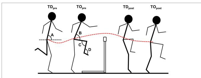
FIGURE 2 | Representative schematic of the four critical instants used in the current study (TD<sub>pre</sub>, TO<sub>pre</sub>, TD<sub>post</sub>, and TO<sub>post</sub>). Bold segments represent segments analyzed. Angles analyzed are represented with A (trunk angle), B (hip angle), C (knee angle), and D (ankle angle). Red, dashed line represents center of mass path.
