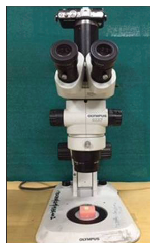
Figure 4: Testing nature of bond failure under stereomicroscope
