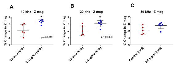
**Figure 2.** Percentage changes in impedance magnitude (Z mag) with pLDH. Functionalized interdigitated electrode (IDE) sensors were incubated with 2.5 ng/mL pLDH in phosphate-buffered saline (PBS) and non-spiked PBS at measurement frequencies (**A**) 10 kHz, (**B**) 20 kHz, and (**C**) 50 kHz. Error bars are standard deviation, \* indicates  $p \le 0.05$  (Welch's t-tests).
