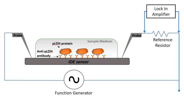
**Figure 1.** Circuit model and measurement setup used for detection of *Plasmodium* lactate dehydrogenase (pLDH). The cross-sectional view of the measurement setup illustrates detection of spiked pLDH protein in a sample medium with the sensing area. Probe electrodes were placed to deliver excitation current to, and to measure electrical signals from, the sensors.
