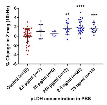
**Figure 3.** Aggregate data of percentage changes in impedance magnitude (Z mag) with increasing concentrations of pLDH in PBS. Percentage change impedance of with non-spiked PBS (control), 2.5 pg/mL, 25 pg/mL, 250 pg/mL, 2.5 ng/mL, and 25 ng/mL of pLDH, at a measurement frequency of 10 kHz. Error bars are standard deviation, \*\*  $p \le 0.01$ , \*\*\* p < 0.001, \*\*\*\* p < 0.0001 compared to control (Dunnett's test).
