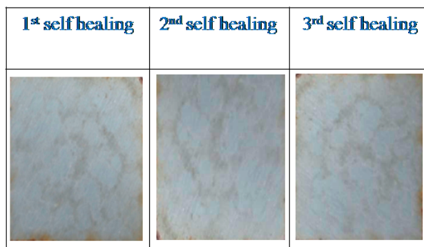
Figure 4. Typical photographs of exposed PU-11-3-3-CeO 2 -P-Healed coating.
