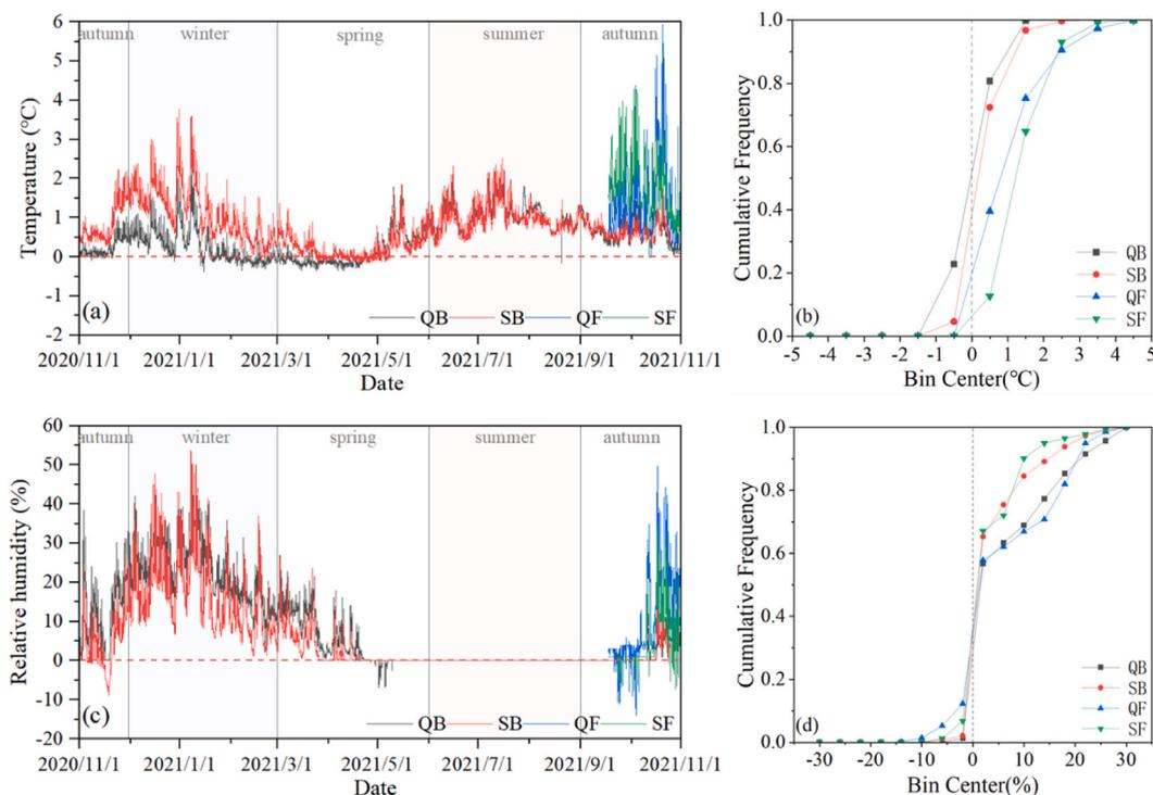
**Fig. 6.** Fluctuations and cumulative frequency in vertical temperature differences (a,b) and relative humidity (c ~ d) in the front and back chambers. The temperature differences ranged from  $-5$  to  $5$  °C in 10 intervals (1 °C per interval) and the humidity differences ranged from  $-32\%$  to  $32\%$  in 16 intervals (4% per interval). (the vertical difference =  $h_{3.0} - h_{0.1}$ ).
