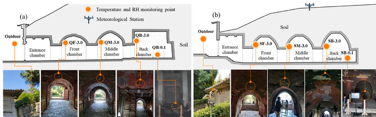
**Fig. 3.** The monitoring plan for the two tombs of the Southern Tang Dynasty: (a) Qinling Tomb; (b) Shunling Tomb. The monitoring point is indicated by the chamber name and the monitoring height, such as “QF-3.0”.
