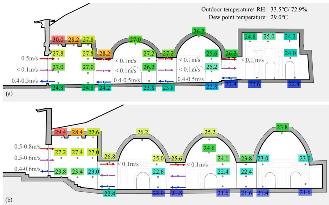
Fig. 9. Measured surface temperature of the walls and air velocity in (a) the Qinling Tomb and (b) the Shunling Tomb at 15:30 on July 11, 2021.
