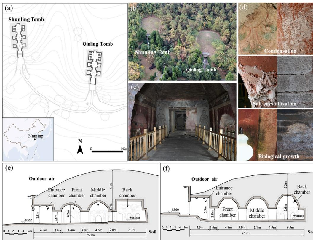
**Fig. 1.** Introduction of two tombs of the Southern Tang Dynasty: (a) location of the tombs; (b) view of the tombs; (b) stone sculptures in the Qiling Tomb; (d) the representative diseases, namely condensation, salt crystallization, and biological growth; (e) cross-section of the Qiling Tomb; (f) cross-section of the Shunling Tomb.
