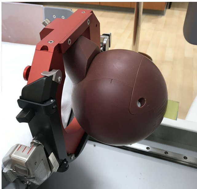
FIG. 2. Relative output factors measurement setup using film inside the Solid Water phantom.
