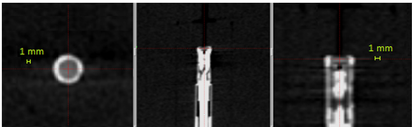
FIG. 4. Cone beam computed tomography CBCT of the MicroDiamond detector and centering it at the unit center point.
