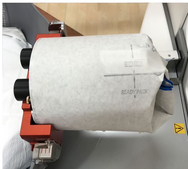
FIG. 3. The CATPHAN phantom wrapped in a radiographic film for the source counting measurement.
