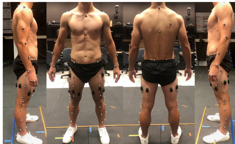
Figure 1. Delsys Trigno sensor and retroreflective motion capture marker placement.
