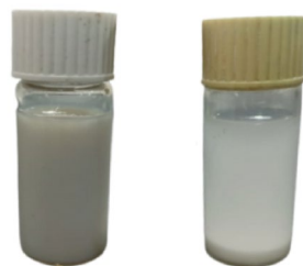
Fig. 1. Two samples of dispersion treated and untreated \text{nAl}_2\text{O}_3 after 20 days.
