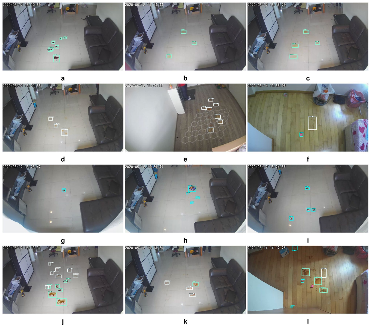
Figure 5. Real-time detection of stain, foot stain, trash.
