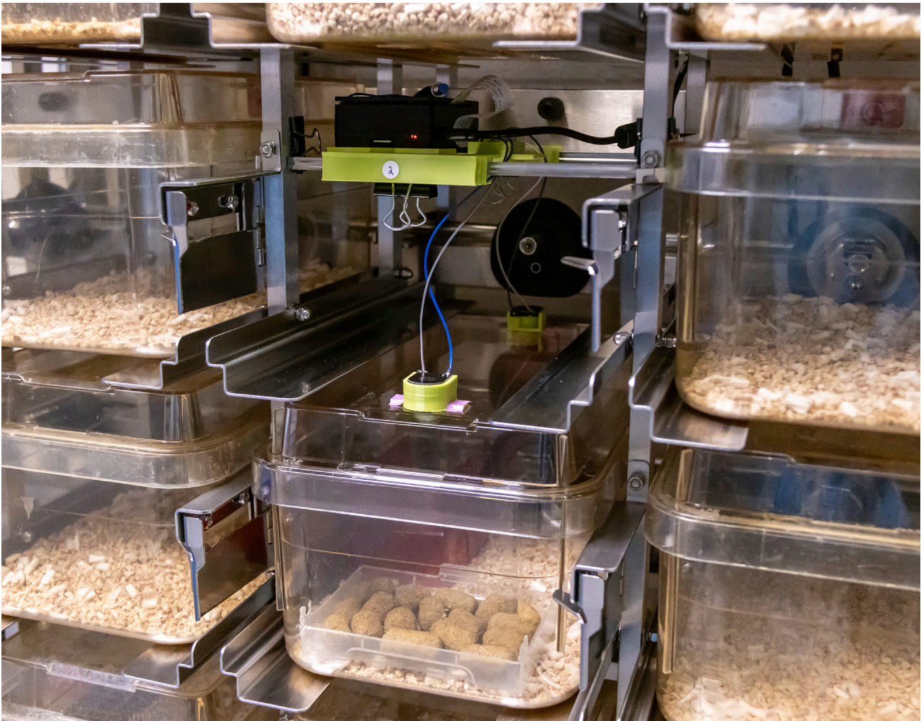
Figure 4. The Home-Cage Camera System hardware mounted in a standard mouse rack The camera preview shown in Figure 2 was recorded with the equipment in the position shown here.
