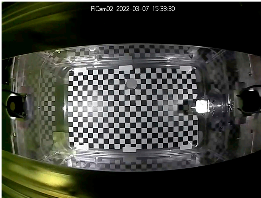
Figure 6. A frame from a day-time video showing a 1 cm checkerboard pattern on the bottom of an empty home-cage. HCCS_1cm_checkerboard.png was printed, trimmed to size, and taped in position. This pattern may be used to determine the real-world scale of your video and assess the need for image distortion correction.
