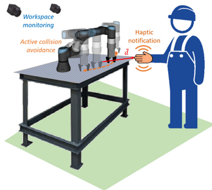
Figure 4. The concept of improved HRC combines principles of active collision avoidance with an increased awareness provided by the wearable haptic feedback device.
