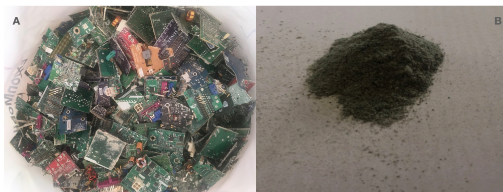
Figure 1 PCB disassembled and crushed. (A) PCBs disassembled, 3 × 3 cm manually cut pieces. (B) PCB crushed for bioleaching assays final size 250 μm.
