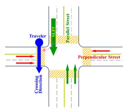
**Fig 1. Layout of a cross street intersection and traffics.** The traveler is standing at the street corner indicated by the blue circle and intends to cross the perpendicular street in the direction indicated by the blue arrow. Red and green arrows are perpendicular and parallel traffic, respectively. The near lane parallel traffic (thick green arrow, NLPT) comes from behind, over his left shoulder. Right-turn cars (magenta dashed arrow) may share the near lane.
