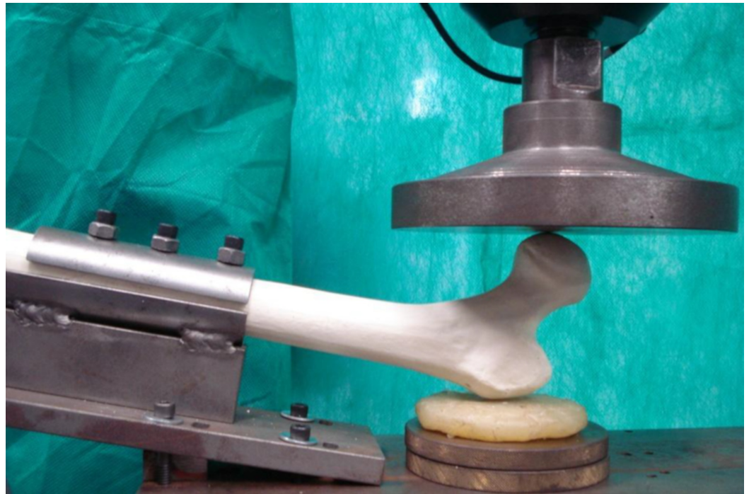
FIGURE 2: Femur adjusted on the device during test
