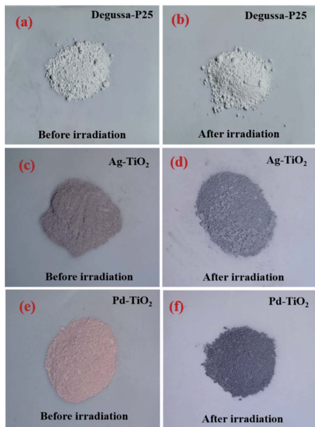
Fig. 10 (a)–(f) represent the photochromic effect in Degussa-P25, Ag + doped TiO 2 , and Pd 2+ doped TiO 2 , respectively.
