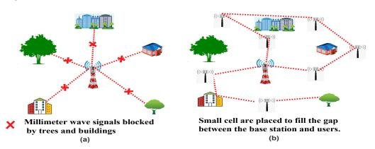
the small cell can be placed at a short distance to transmit the signals easily, as shown in Figure 7b.
