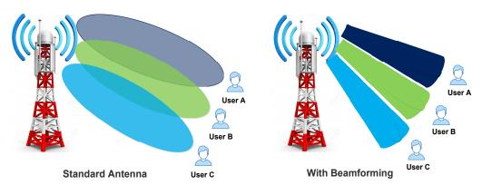
Figure 8. Pictorial Representation of communication with and without using beamforming.
