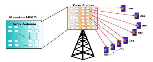
Figure 2. Pictorial representation of multi-input and multi-output (MIMO).
