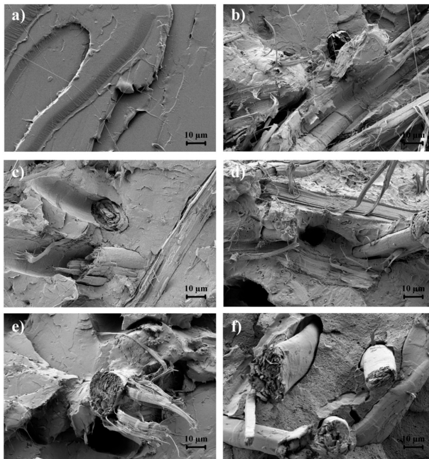
Figure 4. Field emission scanning electron microscopy (FESEM) images of the fracture surfaces of the polylactide (PLA)/flaxseed fiber (FF) pieces of: (a) PLA; (b) PLA/FF; (c) PLA/FF + (3-glycidyloxypropyl) trimethoxysilane (GPTMS); (d) PLA/FF + epoxy-based styrene-acrylic oligomer (ESAO); (e) PLA/FF + poly(styrene-co-glycidyl methacrylate) (PS-co-GMA); (f) PLA/FF + maleinized linseed oil (MLO). Images were taken at 1000× with scale makers of 10 µm.
