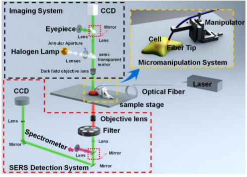
Figure 1. The schematic diagram of the micromanipulation-Raman detection system. Adapted with permission from [80] Copyright 2019 Elsevier B.V.
