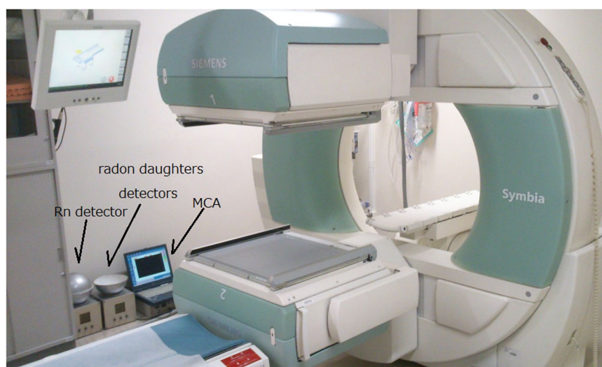
Figure 7. Photo during measurements of Rn-222 concentration and daughter radionuclides of Rn-219 and Rn-222 with energy spectra.
