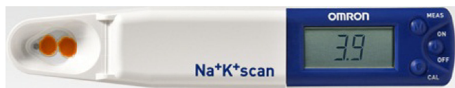
Figure 2. Self-monitoring device used in the randomized trial. Portable handy-sized urinary Na/K ratio monitor (HEU-001F, OMRON Healthcare Co., Ltd., Kyoto, Japan) used for self-monitoring of the dietary lifestyle of the participants during the randomized trial. This device measures urinary Na and K concentrations, and calculates urinary Na/K ratio via ion selective electrodes. Only participants in the “device + usual care” intervention group were given the monitoring device. These participants were then asked to measure at least one spot urine Na/K ratio daily.
