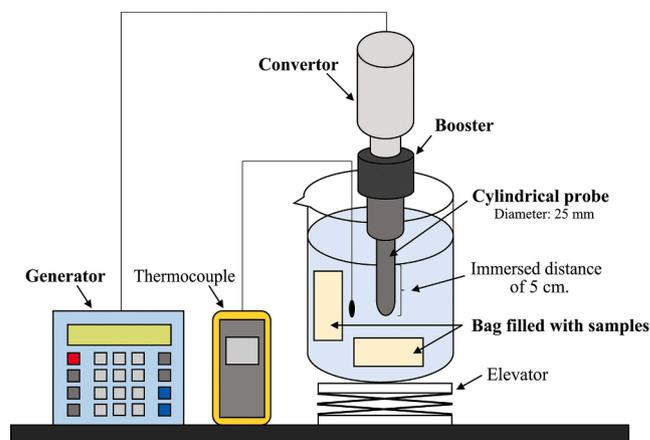
Fig. 1. Schematic diagram of ultrasound set up.
