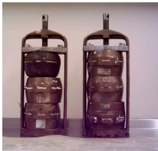
Figure 3. Conventional two-part brass flasks used in dental laboratories.
