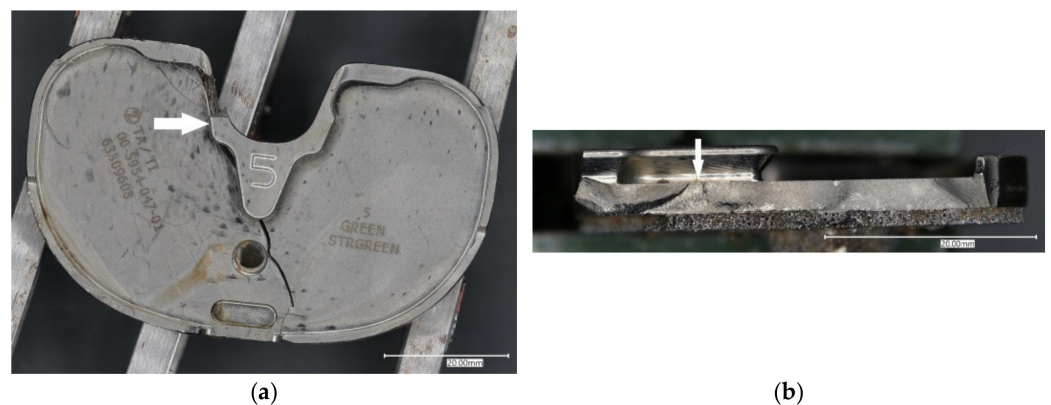
Figure 6. Microphotographs depicting signs of a fatigue fracture of the tibial tray with fatigue crack initiation site (arrows) viewed from above (a) and from the fracture side (b).
