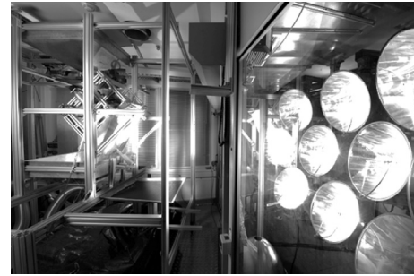
Fig. 4. The Cologne high-flux solar simulator of the German aerospace center under operation.
