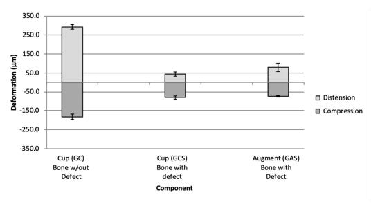
**Figure 3.** Bar graph of mean elastic deformation (distension and distension) of GC (no bony defect; scenario 1) and GCS and GAS (with bony defect; scenario 2).
