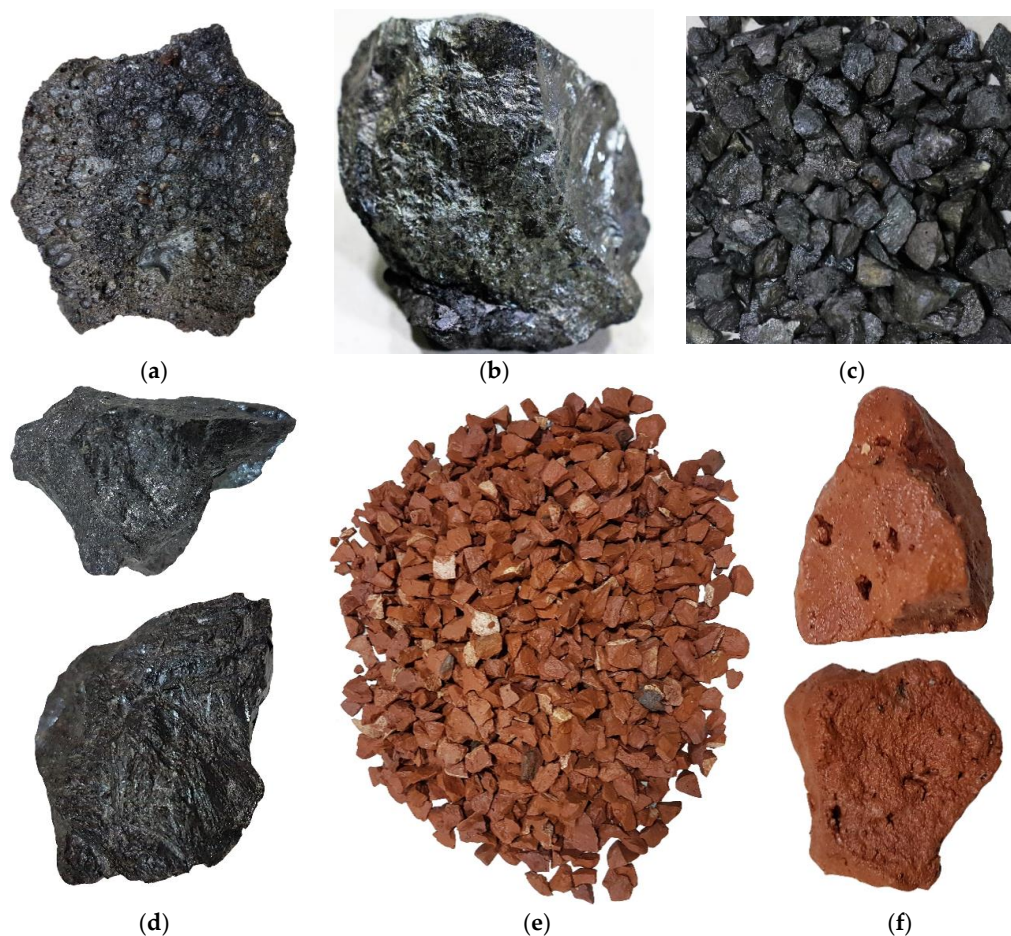
Figure 1. Induction furnace steel slag boulders: (a) steel slag with more void, (b) steel slag with less void; steel slag aggregate (SSA): (c) steel slag coarse aggregate, (d) close view of SSA; brick aggregate (BA): (e) brick coarse aggregate, (f) close view of BA.
