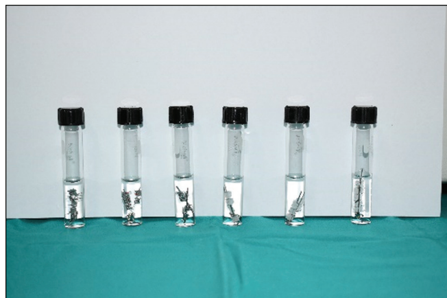
Figure 3: Simulated orthodontic appliances immersed in artificial saliva for cytotoxicity assessment
