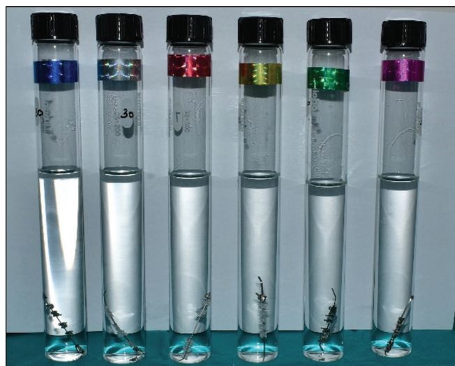
Figure 2: Simulated orthodontic appliances immersed in artificial saliva for quantitative assessment
