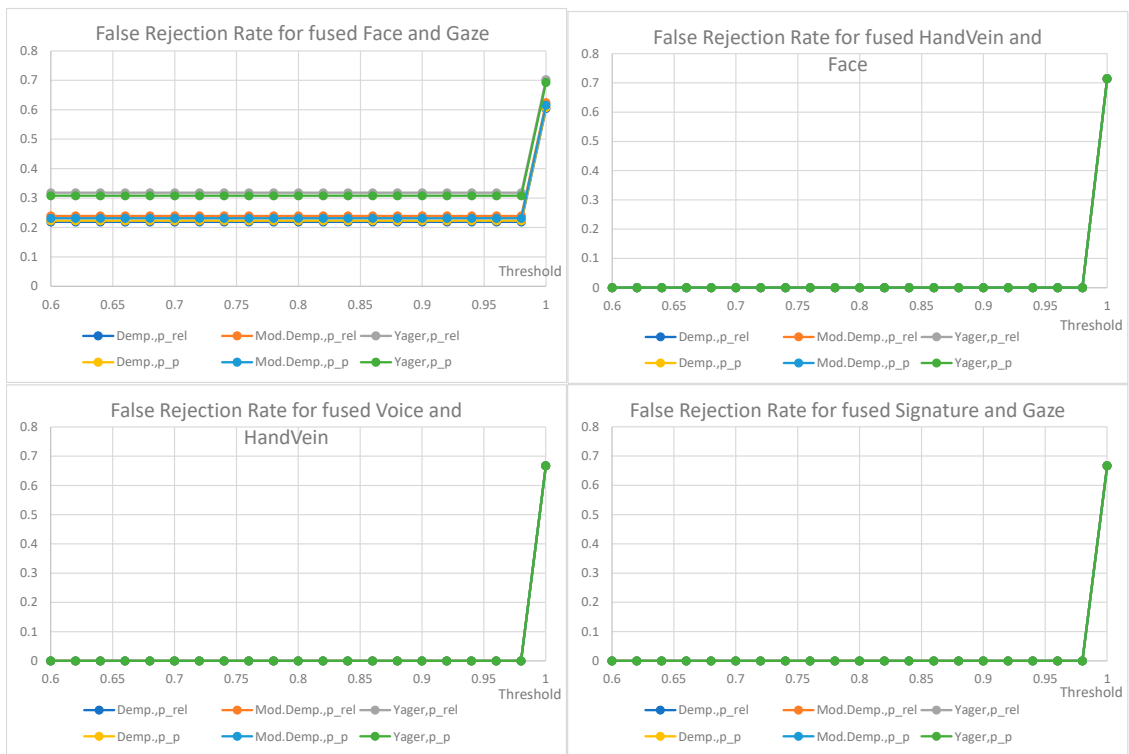
Figure 13. FRR for the fusion of face and gaze (13 pairs), FRR for the fusion of hand vein and face (7 pairs), FRR for the fusion of voice and hand vein (6 pairs), FRR for the fusion of signature and gaze (6 pairs). All other values are the same when a single curve is visualized.
