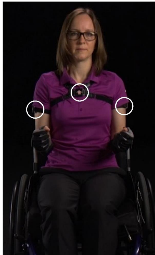
Figure 2. Three inertial measurement units (IMU) were secured to all participants on both of their lateral arms and their chest using elastic straps. The circles indicate where the IMUs are attached. Note: The individual pictured is study staff and not a research participant.
