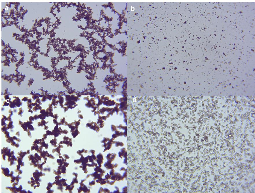
**Fig. 5.** (a)  $800\times$  optical microscope image of citrated  $\text{Fe}_3\text{O}_4$ . (b) Same magnification of TEOS functionalized silica surface beads used in this assay. (c) Commercial Zymo product. (d) Silica surface beads prepared by another method based on seed polymerization described in Section 2.4. Aggregation is observed in samples (a) and (c).
