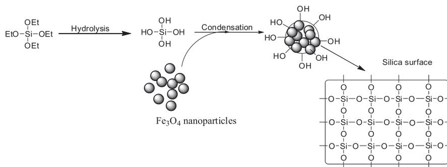
**Fig. 1.** Formation of Silica surface on  $\text{Fe}_3\text{O}_4$  nanoparticles with TEOS.
