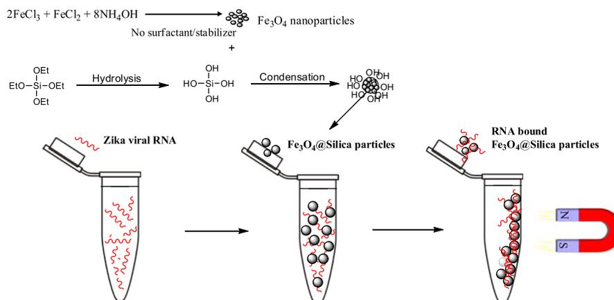
**Fig. 7.** Preparation of  $\text{Fe}_3\text{O}_4$ @Silica particles in 1-pot 2-step pathway and workflow of Zika viral RNA extraction with magnetic separation.
