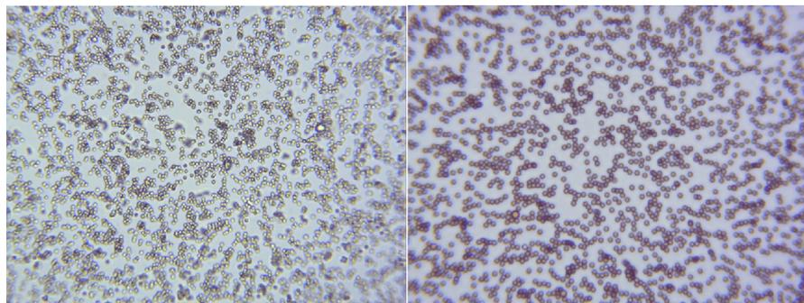
**Fig. 4.**  $800\times$  magnification of microscopic images to illustrate the well-defined spherical shape and monodispersed size: in-house silica coated polymer microparticles (left); reference 2.8–2.6  $\mu\text{m}$  Dynabeads® (right).
