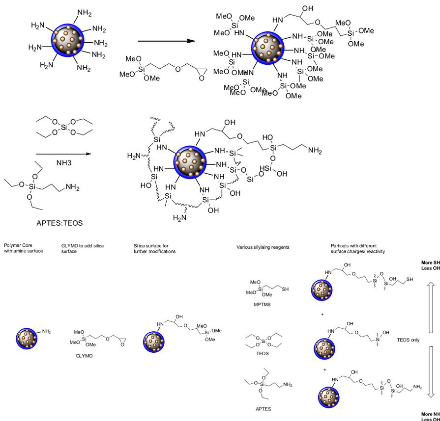
**Fig. 3.** Preparation of silica surface spherical monodispersed microparticles (polymer based), and the additions of variable MPTMS, TEOS, APTES for modified silica surface with different surface charges and reactivity.
