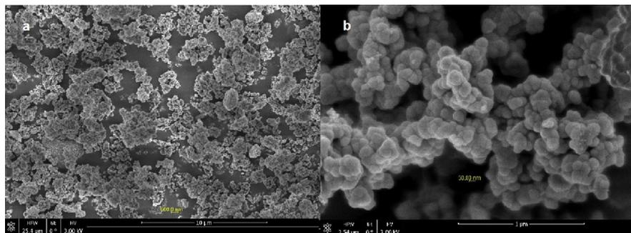
**Fig. 6.** (a) SEM analysis of  $\text{Fe}_3\text{O}_4$ @Silica with 500 nm & 10  $\mu\text{m}$  scales. (b) SEM analysis of  $\text{Fe}_3\text{O}_4$ @Silica with 50 nm & 1  $\mu\text{m}$  scales.
