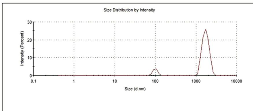
**Fig. 2.** Dynamic light scattering (DLS) size measurements of  $\text{Fe}_3\text{O}_4$ @Silica particles with 55% silica mass ratio (TEOS:NP, 4:1 w/w) was obtained using a Malvern ZETASIZER NANO ZSP. Z-average diameter =  $1.77$   $\mu\text{m}$ , PDI = 0.370, Peak 1 =  $1.75$   $\mu\text{m}$  (91.1%), Peak 2 =  $0.099$   $\mu\text{m}$  (8.9%).
