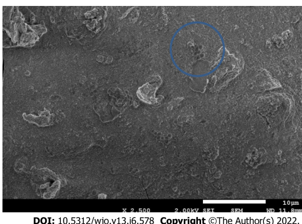
Figure 5 Bacteria inside the lumps formed by electrocoagulation of the medium.
