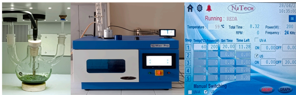
Fig. 1. Sonication-assisted microwave (NuWav- Pro/N \mu Tech, India).
