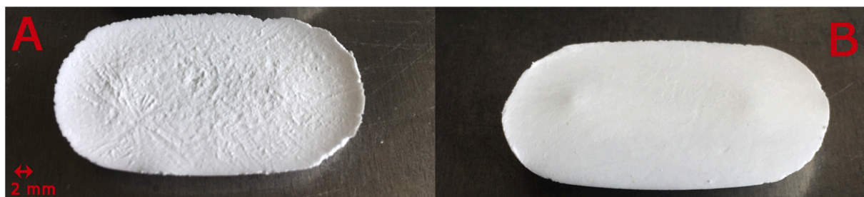
Fig. 4. Picture of the (A) optimized low-dose and (B) high-dose ODT. A skin effect is visible on the low-dose tablet.
