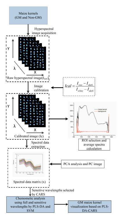
**Figure 2.** Flowchart of image processing and data analysis for discrimination of genetically-modified (GM) maize kernels. CARS: competitive adaptive reweighted sampling; PLS-DA: partial least squares discriminant analysis; ROI: region of interest; SVM: support vector machine.
