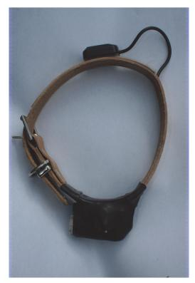
Fig 1. The GPS collar. The battery compartment, GPS and logger with external toggle switch all positioned ventrally and a movable GPS antenna located dorsally.
