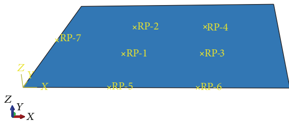
FIGURE 5: The initial fixture locating layout of the aluminum alloy sheet metal part.
