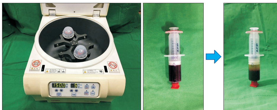
Fig. 1. Leukocyte-poor platelet-rich plasma (LP-PRP) Arthrex ACP platelet separation system. Blood (13.5 mL) and anticoagulant citrate dextrose solution A (ACD-A, 1.5 mL) were mixed and transferred into a double ACP syringe and centrifuged at 380 \times g (1,500 rpm) for 5 minutes to separate the red blood cell/leukocyte and plasma-platelet layers, the latter of which was collected as LP-PRP (about 4 mL).
