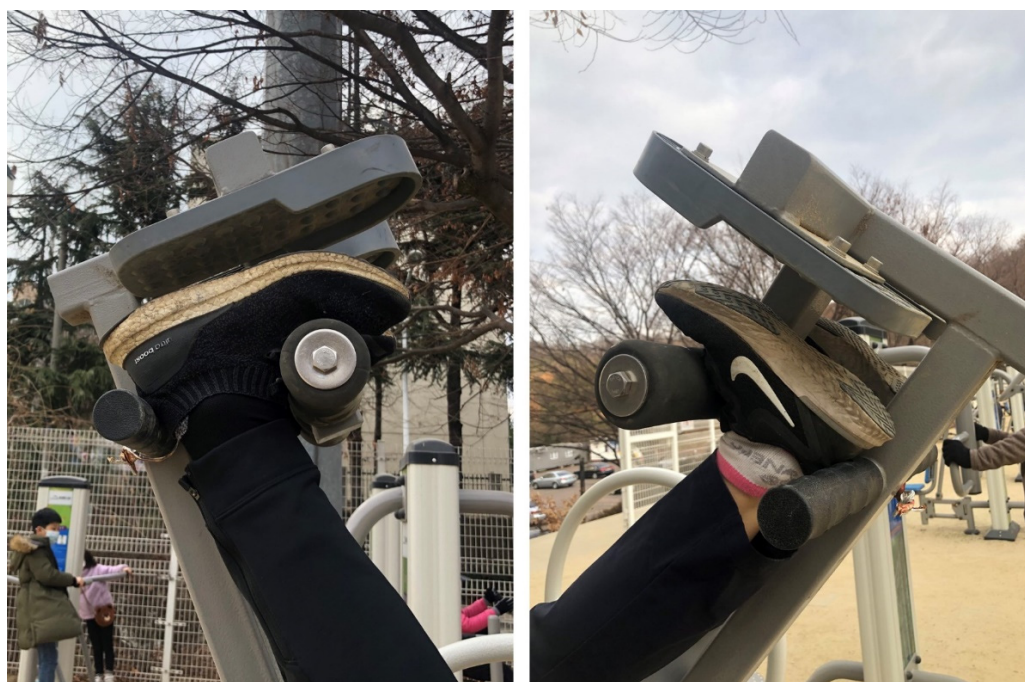
Figure 3. Single-pin ankle lock design is commonly found in public devices.
