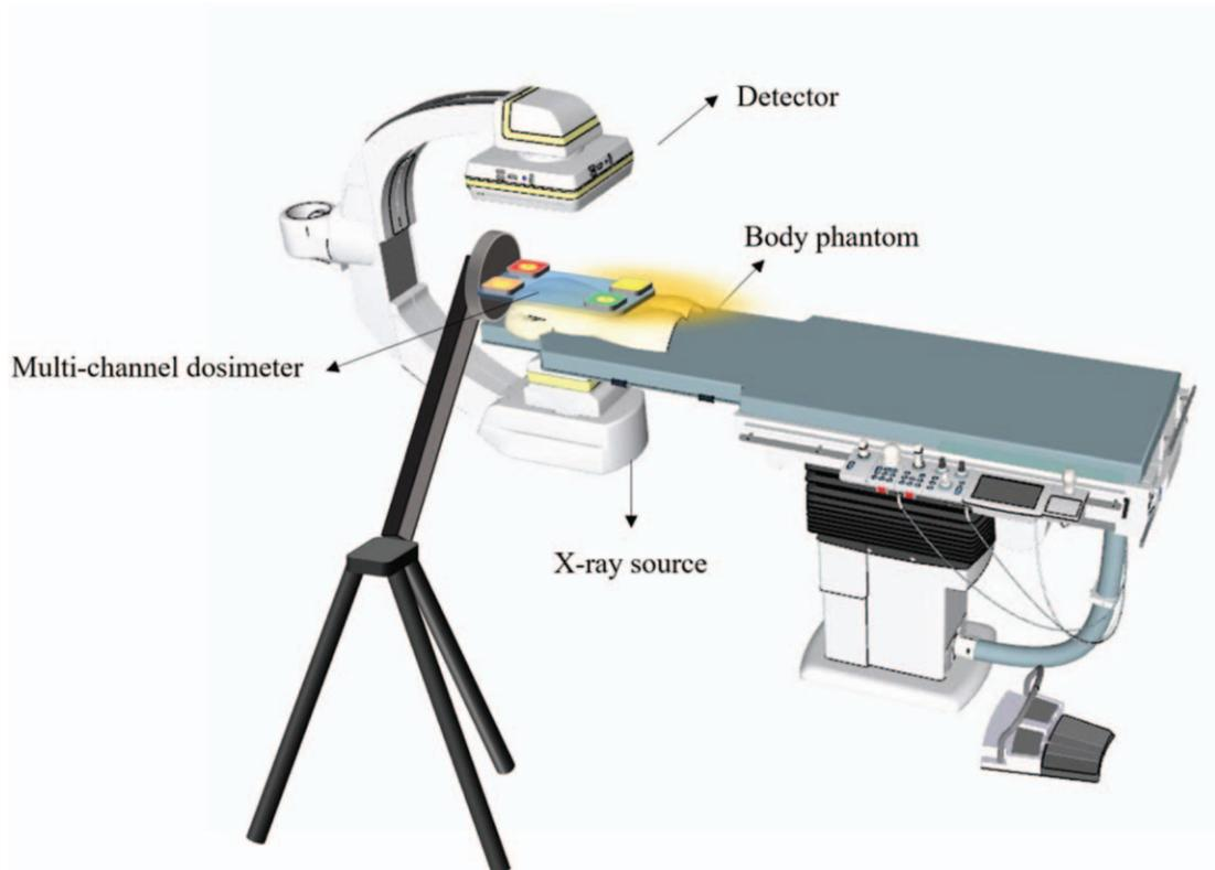
**Figure 1.** The chest phantom was laid on the operating table 50 cm above the X-ray tube. The fluoroscopic image was focused on the xiphoid process. Real-time radiation exposure data were collected using a commercially available multi-channel dosimetry system.
