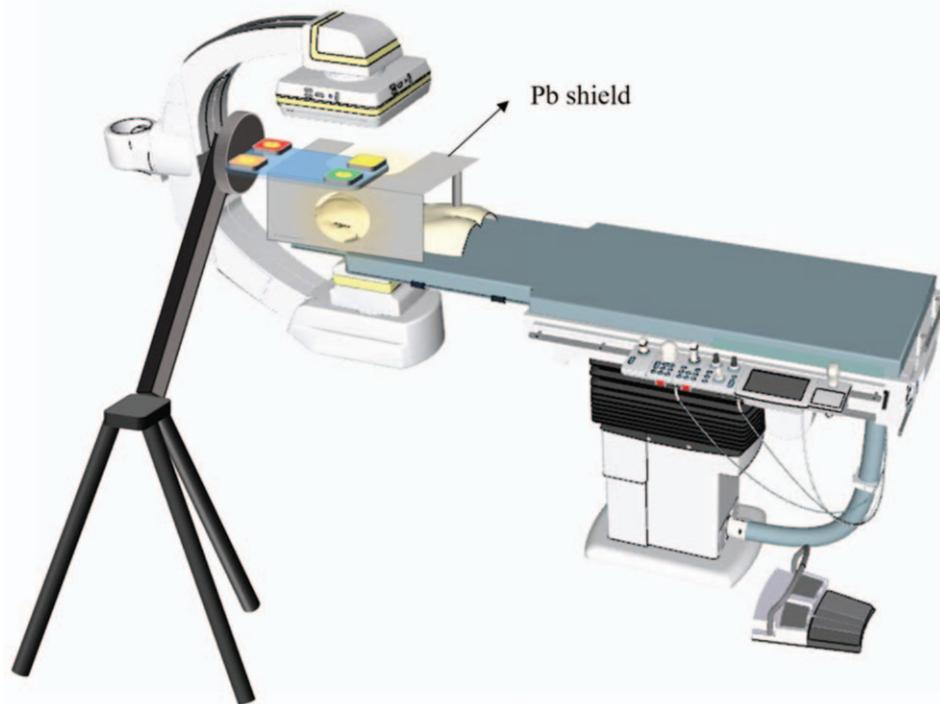
**Figure 3.** A photographic depiction of the relationship between the chest phantom, shielding device, and the C-arm controller. The C-arm is in the inverted configuration.
