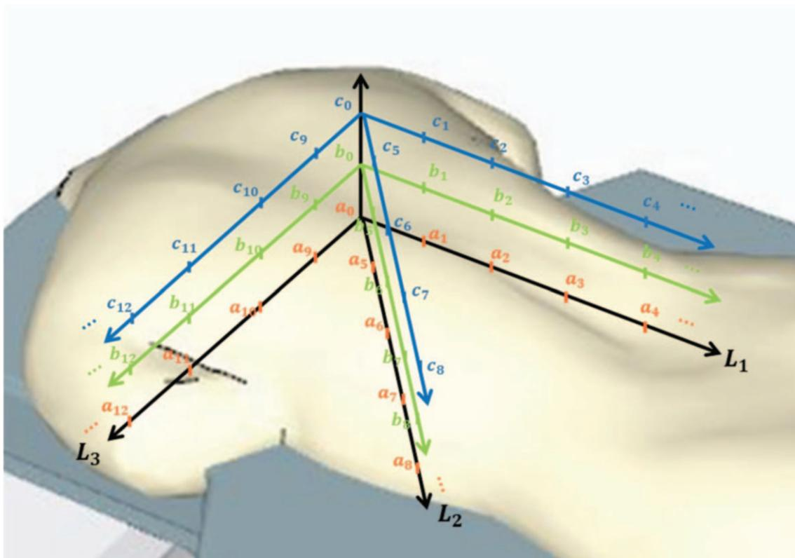
**Figure 2.** Air kerma rates as scatter radiation doses were collected at horizontal distances of 0 cm, 10 cm, 20 cm, and 30 cm from the xiphoid process of the chest phantom at 3 angular positions of 0° (L1), 45° (L2), 90° (L3), and 3 height planes, that is, 0 cm (A), 5 cm (B), and 10 cm (C). Measurements were made at 1, 3, 5, and 10 minutes.
