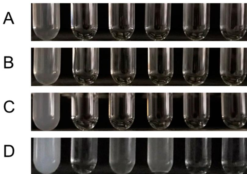
**Figure 3.** Appearance of aqueous solutions of  $\alpha$ -T3DMG with or without TCA.  $\alpha$ -T3DMG concentrations in the test solutions are (A) 2.94 mmol/L, (B) 5.88 mmol/L, (C) 11.76 mmol/L, and (D) 23.52 mmol/L.
