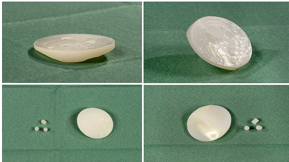
FIGURE 6: Photographs of the failed implant displaying separate implant base and pegs.
