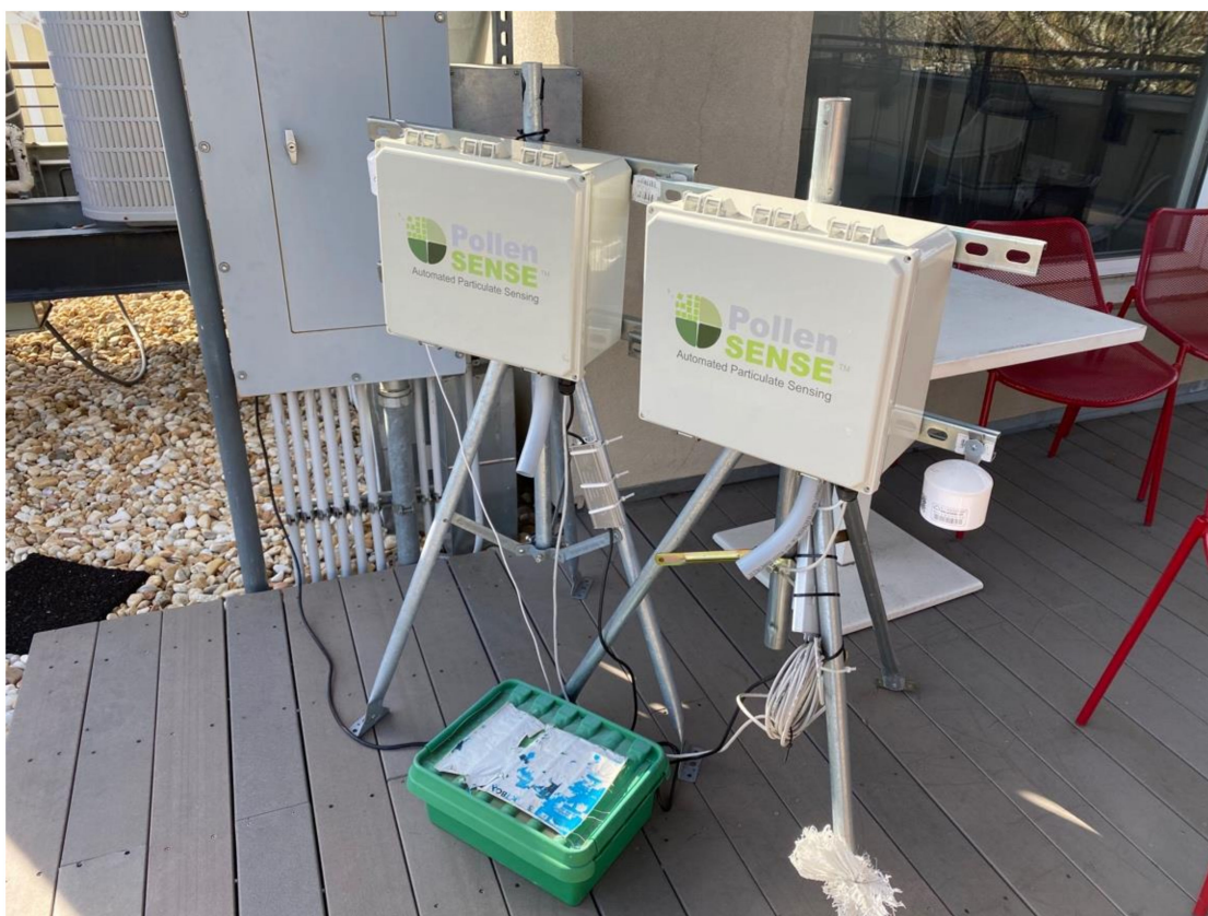
Figure A1. Colocation of two APS-300 sensors at the Southface Site for the internal consistency tests.
