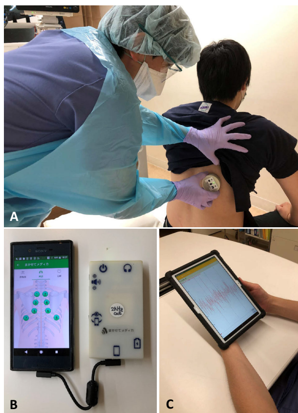
Figure 3. Auscultation method with a novel device. Physicians with PPE apply the wireless stethoscope over the patient's lungs (A), with lung sounds being automatically transferred to the receiver and recorded in an app in the cellular phone (B). Both the receiver and the cellular phone are usually wrapped in plastic. The lung sounds are simultaneously transferred to a cloud server as well and can be shared in real time with the medical staff in the green zone using a cellular phone or tablet-type device.
