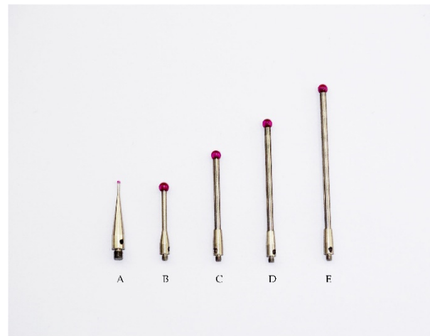
Figure 4. Light pen stylus.
