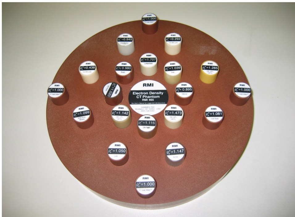
FIG. 1. Electron density CT phantom.
