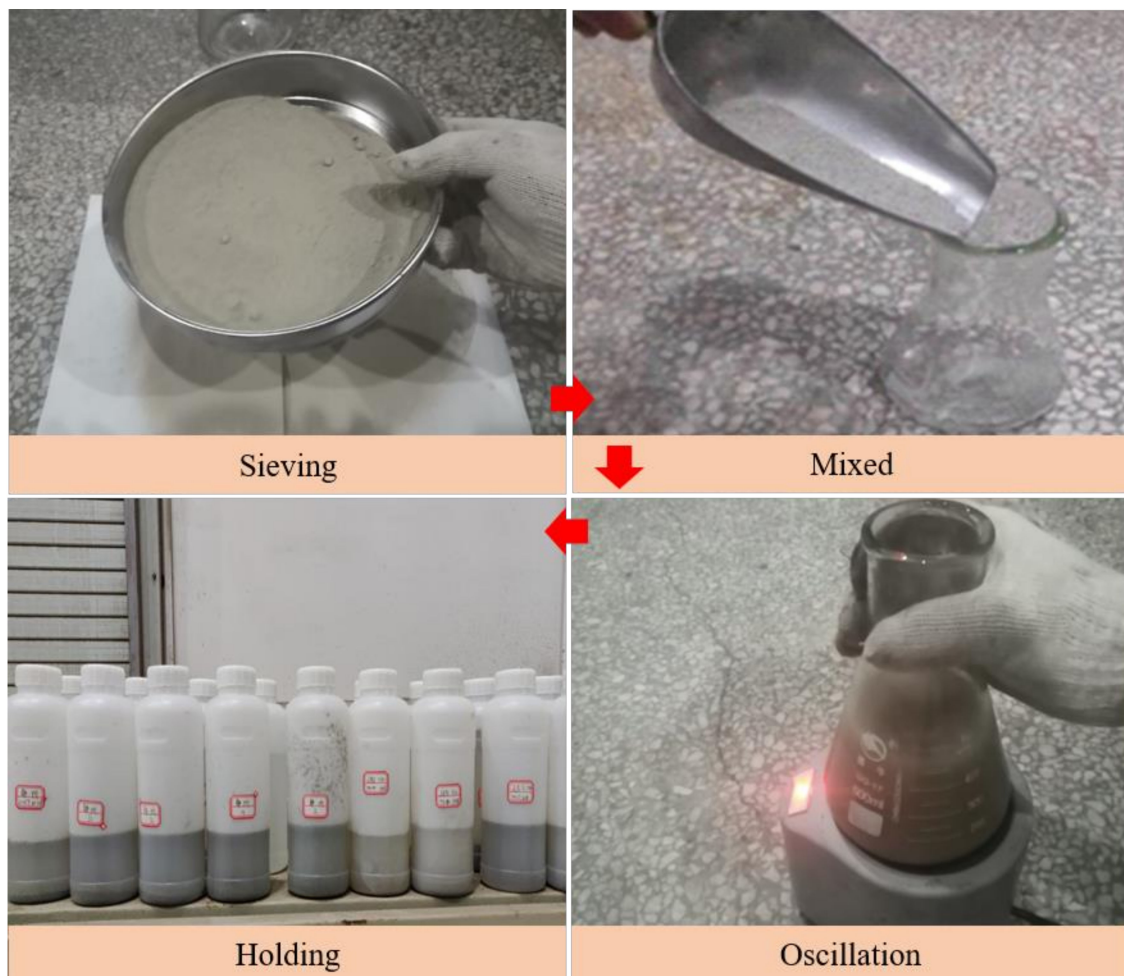
Figure 8. Static leaching test procedure.
