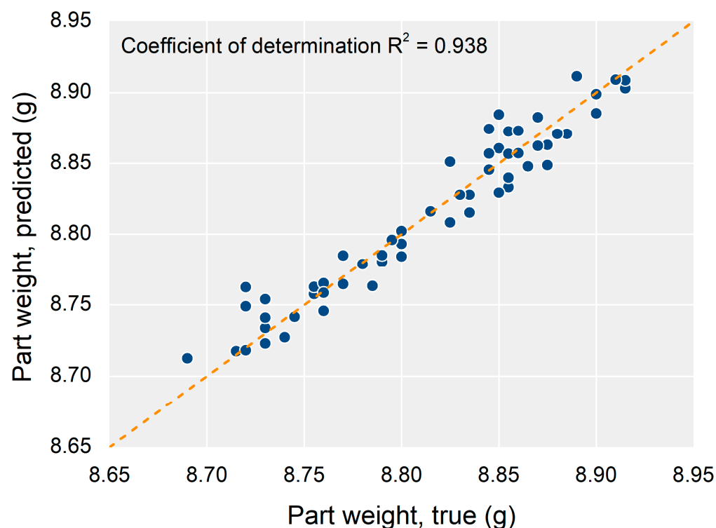
Figure 8. Part weight prediction result by the neural network.
