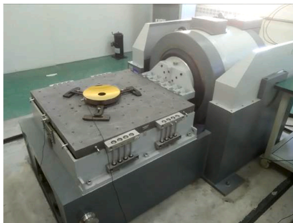
Fig. 14. Dynamics testing of the mirror assembly.
